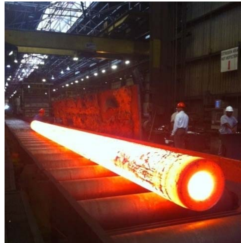
Inconel®740H Pipe after Extrusion at Wyman-Gordon
